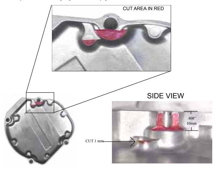
Now that you have cut the cover you also have to cut the gaskets to match. Use the sealing washer (included in the flywheel weight kit) on the cover bolt that goes through the cut area. The 12 ounce weight for the 2002 CR 250 (part number 511) requires using an extra gasket (two gaskets). The 14 ounce weight for the 2002 model and the 12 ounce weight for the 2003-2007 model (part numbers 511H or 514H) requires using two gaskets, one on each side of the supplied 1/8th inch plastic cover spacer.
